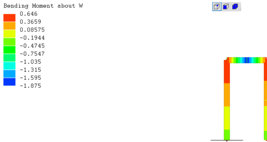
Figure 11 Bending Moment by concentrated force
