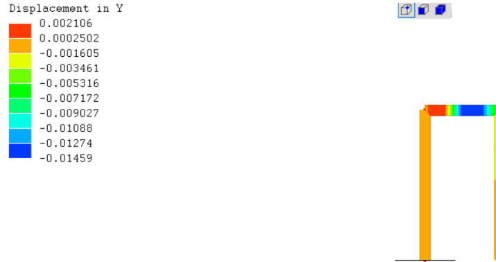
Figure 3 Displacement in Y by concentrated force and distributed force
