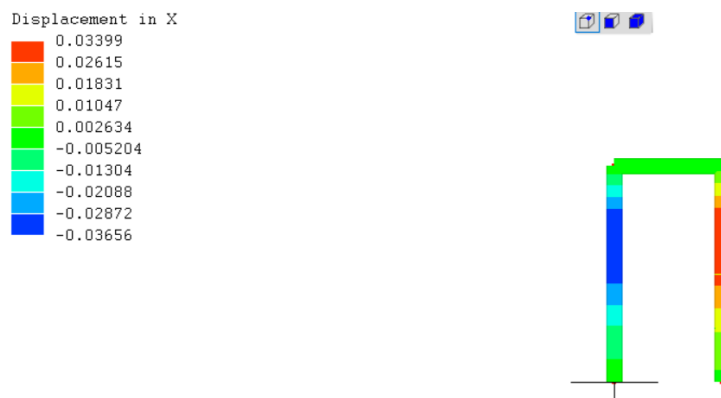
Figure 1 Displacement in X by concentrated force
