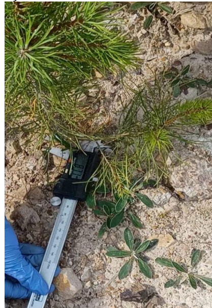
Figure 5 Measurement of the diameter of the saplings with the electronic caliper
