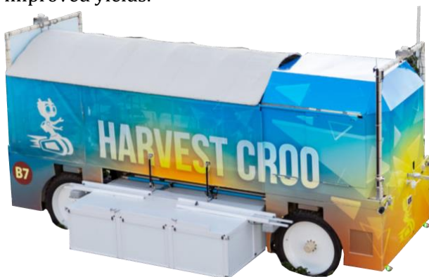
Figure 3 Harvest CROO Robotics' strawberry-picking machine
