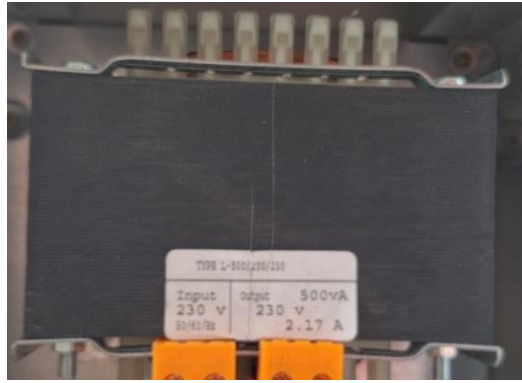
Figure 7 Transformer 230V to 230V with 2A
