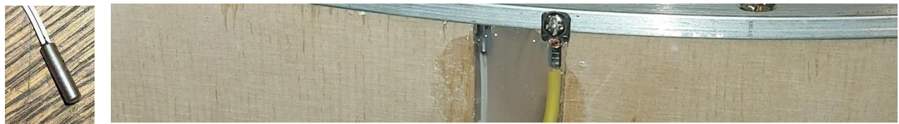
Figure 6 The temperature probe in the aluminum strip
