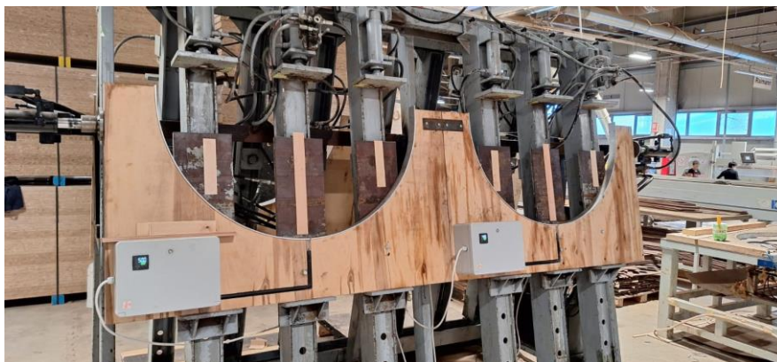
Figure 12 The hydraulic press with the proposed solution for the templates
