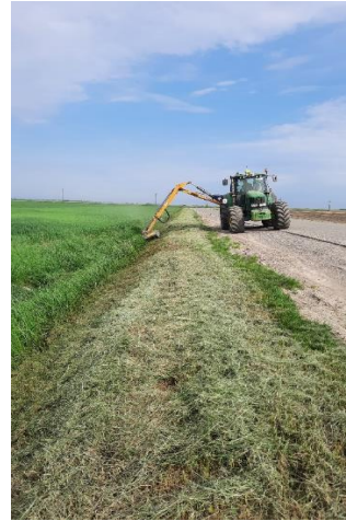
Figure 3. Vegetation cleaning with the chopper on the arm - Photo Marin Ilca
