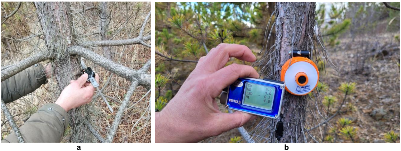
Figure 4 Diameter measurement with a caliper (a) and of the tree height with HaglÖf Vertex 5 Hypsometer (b)
