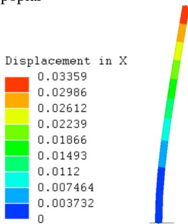
Fig.1 Spindle deformation - poplar
