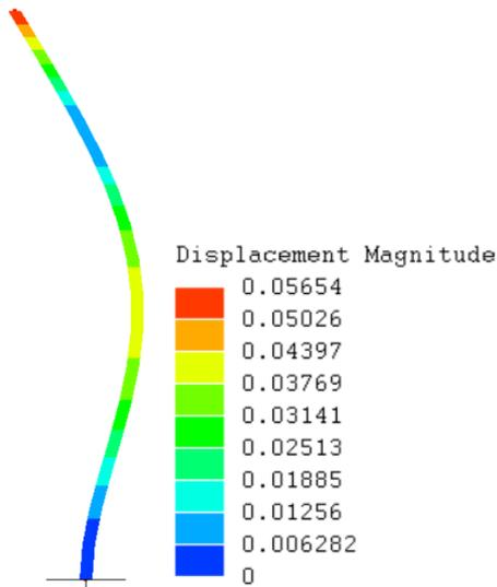
Fig.10 Deformation and displacements of the canopy - poplar
