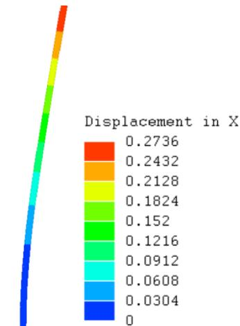
Fig.12 Deformed and displacements of the spindle - fir
