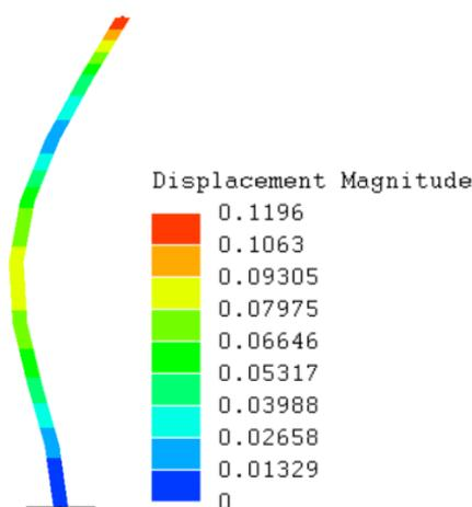
Fig.7 Deformed and displacements of the spindle - poplar
