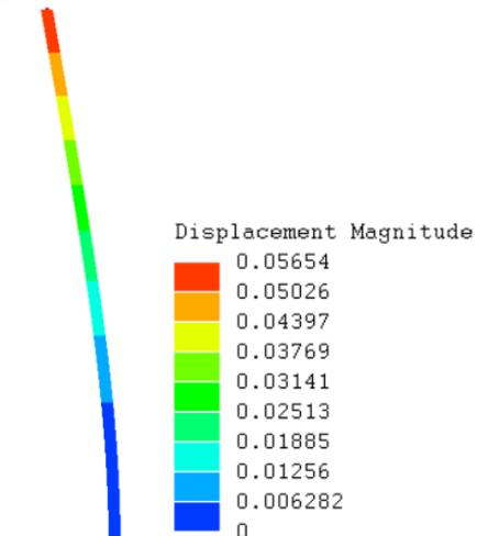
Fig.9. Deformation and displacements of the canopy - poplar
