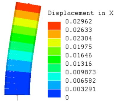
Fig.13 Deformed and displacements of the crown - fir tree
