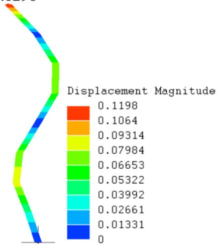
Fig.8 Deformed and displacements of the spindle - poplar
