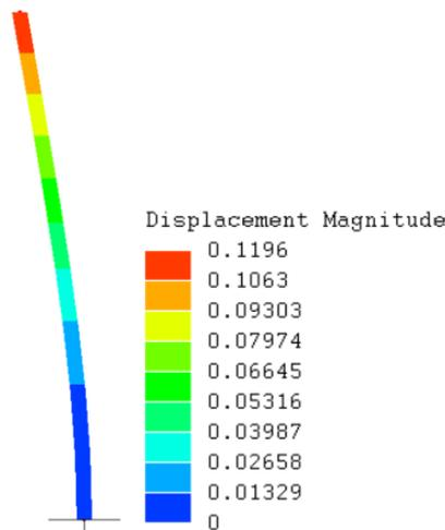
Fig.6. Deformed and displacements of the spindle - poplar
