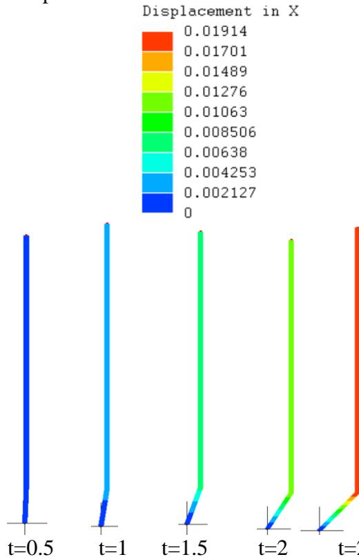
Fig.14 Deformed and displacements of the spindle - fir
