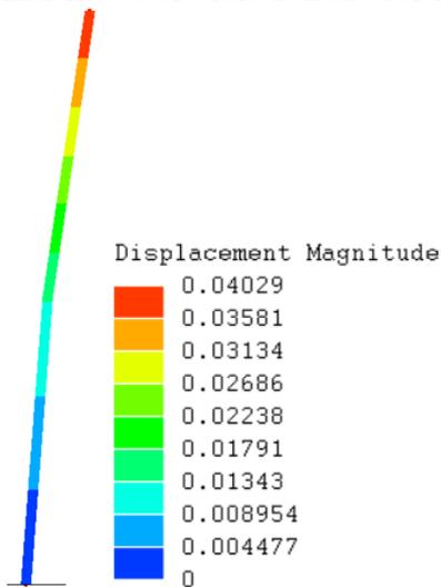
Fig.16 Deformed and displacements of the crown - fir tree
