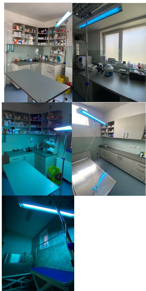
Fig. 3 – Positioning and preparing the UV-C lamp (Original)
