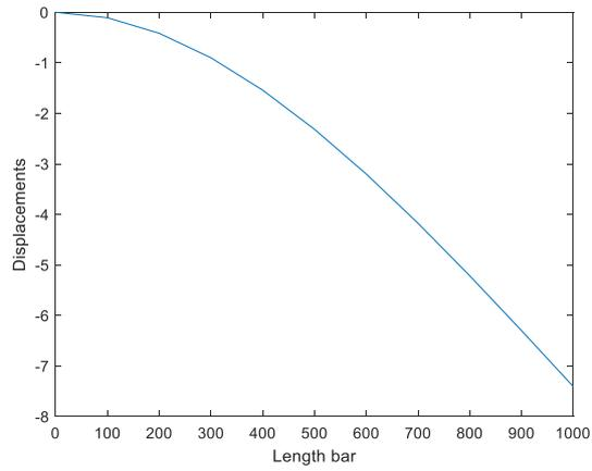
Fig.1 Displacement diagram by Integration method
