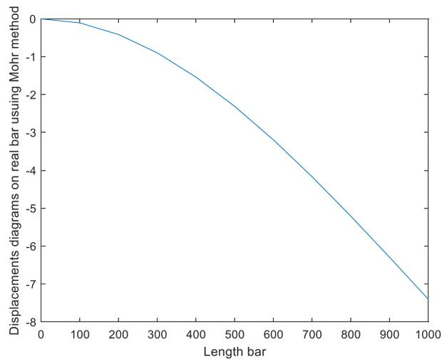
Fig.6 Displacements values along the real beam using Mohr method
