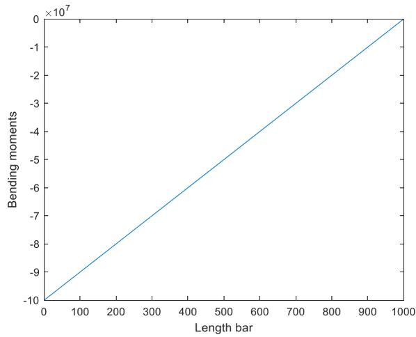
Fig.3 Bending moments diagram using Mohr method
