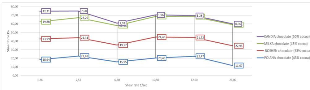
Fig. 2. Comparison of flow curves of melted chocolate samples at 55°C
