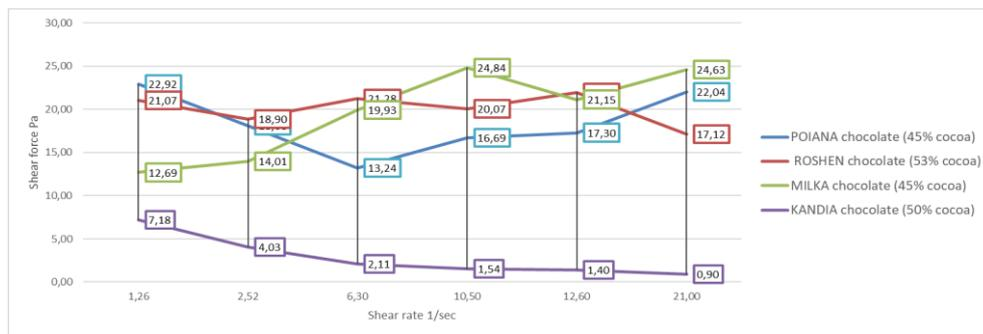
Fig. 1. Comparison of flow curves of melted chocolate samples at 50°C
