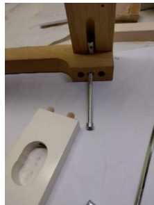
Figure 6 a) Crosspiece with 3 holes to bolt assembly
