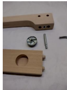
b) Crosspiece with 1 hole to eccentric assembly
