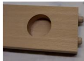
b) Crosspiece with 1 hole to eccentric assembly
