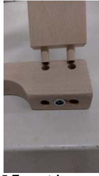
Figure 5 Eccentric assembly without mortises and without bolt channel
