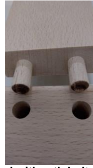
Figure 5 Eccentric assembly without mortises and without bolt channel
