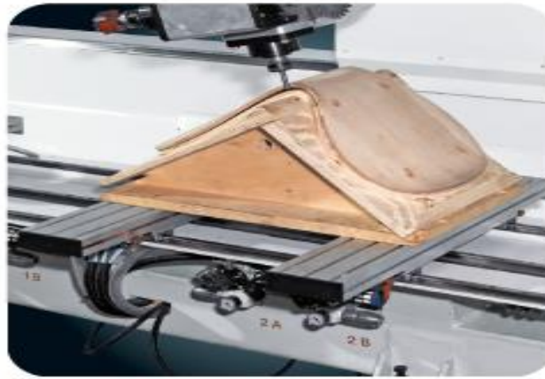
Figure 6 Fixing the landmarks through the vacuum system ( directindustry.com )
