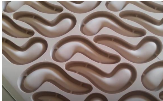
Figure 4 CNC milling (bridge finishing) ( http://www.cnc-3d.ro )
