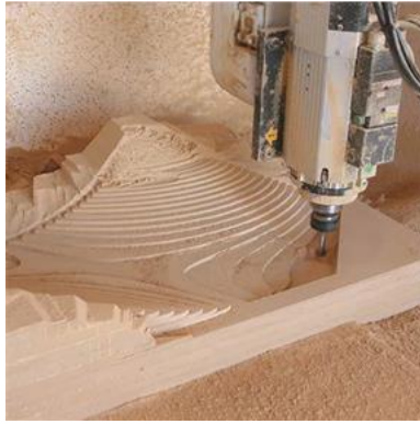
Figure 3 Machining with CNC 5 axes ( tehno-design.ro )
