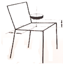
Fig. 9 Impact test against the seat
