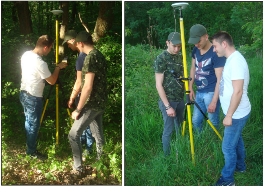
Photo 2 - TRIMBLE R3 receivers used for spatial positioning of details the spatial positioning of the new points was made with the G.P.S. by the static method.
