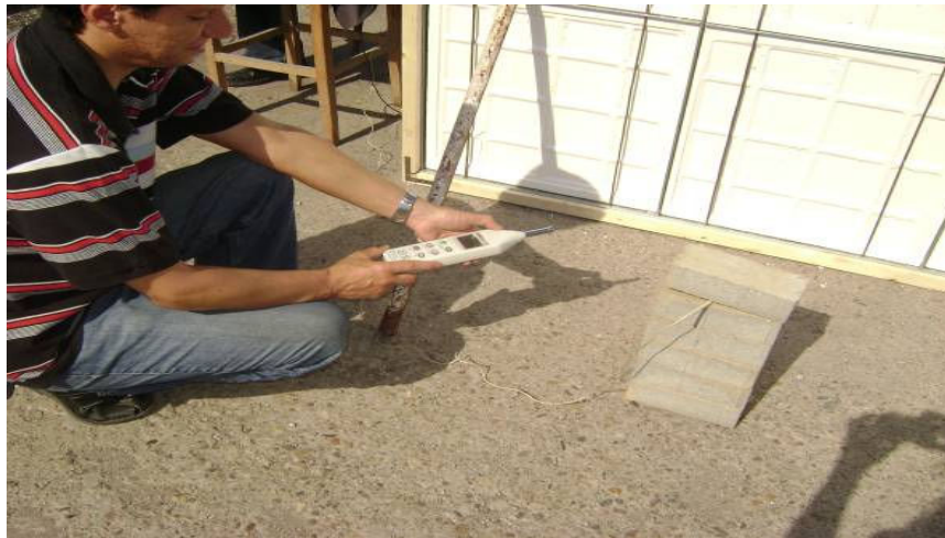
Fig. 2 Measurement of sound-absorbing panels using the test and additional noise recording system in CENTER 332 provided with Digital Sonometer
