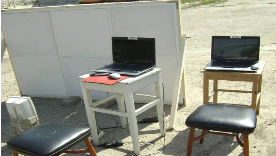
Fig. 2. Installation for testing the behavior of sound-absorbing panels in outdoor environment
