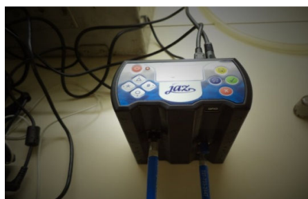
Fig.1. Portable laser spectrophotometer, Jazz from Ocean Optics
