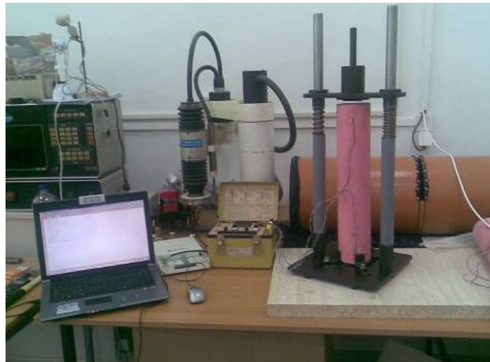
Fig. 3. Laboratory device for determining the modulus of elasticity
