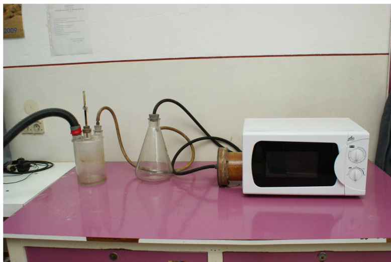
Fig. 1. Microwave with \text{H}_2\text{O} vapor absorption plant
