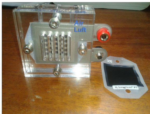
Fig. 4. The fuel cell and the PEM - membrane, Heliocentris
