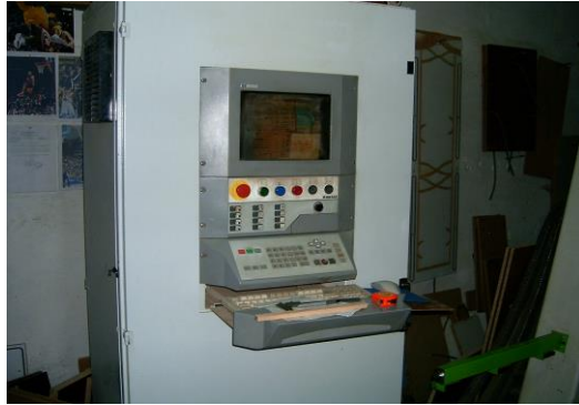
Fig. 1. Control panel vibration control system to HSM ROVER 346.
