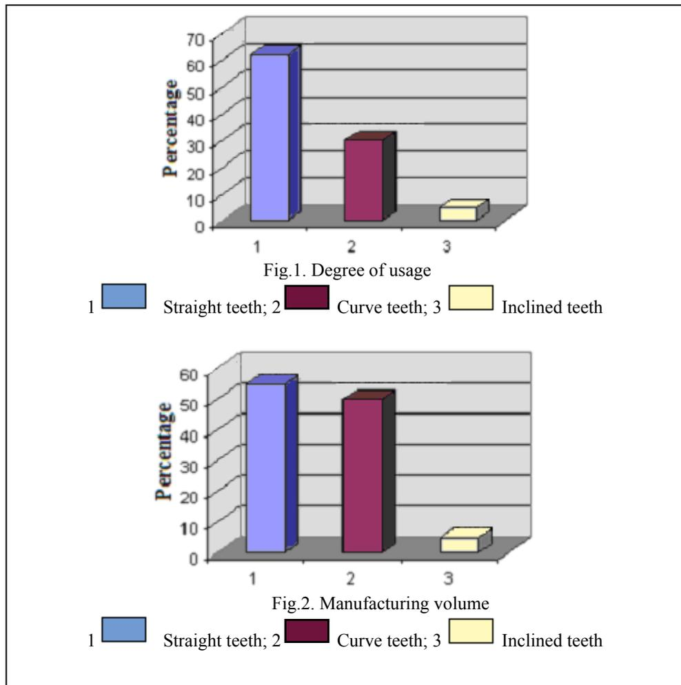
It can be noticed the high frequency of usage of the straight teeth determined by the great number of utilization cases in the machine construction in general as well as for mean of transportation where the number of satellites is greater. Curved conical teeth being used for the main conical gearing (Pantea, I et al. 2008).
