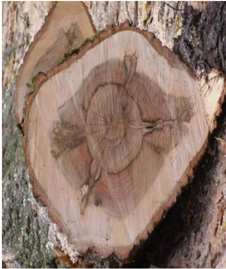
Fig. 2 The frost-crack presence in transversal section on a Turkey oak timber
